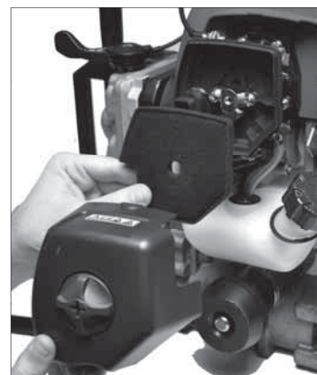
FIG. 27 – FUEL FILTER CLEANING
